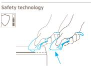
Fully automatic blade retraction – a very high degree of safety
